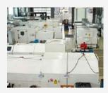
Our numerous dynamometers can simulate any type of braking condition. From a tough mountain descent to E-Bike urban riding, we use them to measure objectively how the brakes perform.
