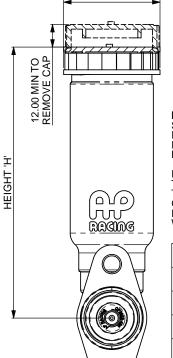
**INLET TYPE 'C'** SELECT MASTER CYLINDER WITH INLET TYPE 'B', PLUS RESERVOIR FROM PART NUMBER CHART BELOW.
