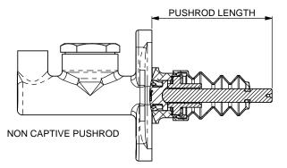
NON CAPTIVE PUSHRODS: CP2623 MASTER CYLINDER IS AVAILABLE WITH NON CAPTIVE PUSHRODS. THIS ENABLES THE REMOVAL OF THE MASTER CYLINDER WITHOUT NEED TO REMOVE THE PUSHROD FROM THE BRAKE PEDAL OR BALANCE BAR ASSEMBLY. PUSH RODS ARE AVAILABLE IN LENGTHS EQUIVALENT TO THOSE SHOWN ABOVE. PUSHROD TYPES:
