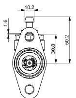
**INLET TYPE 'A'** SELECT MASTER CYLINDER WITH INLET TYPE 'B', PLUS INLET ADAPTOR KIT PART NUMBER CP2623-30
