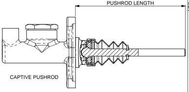
PUSHRODS ARE AVAILABLE IN THE FOLLOWING LENGTHS: 88mm (3.46"), 115mm (4.53") AND 160mm (6.3"). NON-STANDARD LENGTHS AVAILABLE ON REQUEST.
