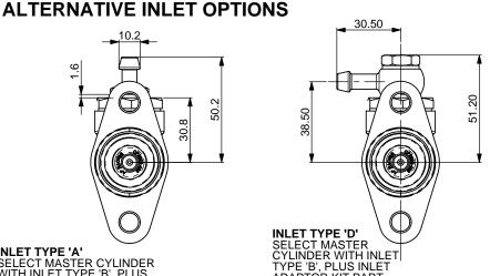
SELECT MASTER CYLINDER WITH INLET TYPE 'B'. PLUS INLET ADAPTOR KIT PART **NUMBER CP2623-41**
